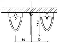
CHROMIUM PLATED DOMICAL GRATING (CODE: 8787Z0) AND CHROMIUM PLATED TOP INLET SPREADER (CODE: 7054Z1), COBRA FLUSH VALVE FJ6000, FIXED ON AND INCLUDING TWO HANGER BRACKETS (CODE: 8127Z0)(URINAL DIVISION. WITH COBRA WATERTECH 32MM CHROME PLATED DEEP SEAL BOTTLE TRAP WITH OUTLET FOR 50MM PVC (CODE: 345/50).
