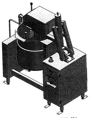
The pot has a torospherical bottom and the steam jacket and is constructed of 3 & 2.5 mm thick 304 stainless steel. About 60% of the pot height is jacketed. The pot has a reinforced rim with a welded-on, trough-shaped pouring lip. It is mirror polished on the exterior and satin finished on the interior surfaces achieved by polishing with successive grits.
