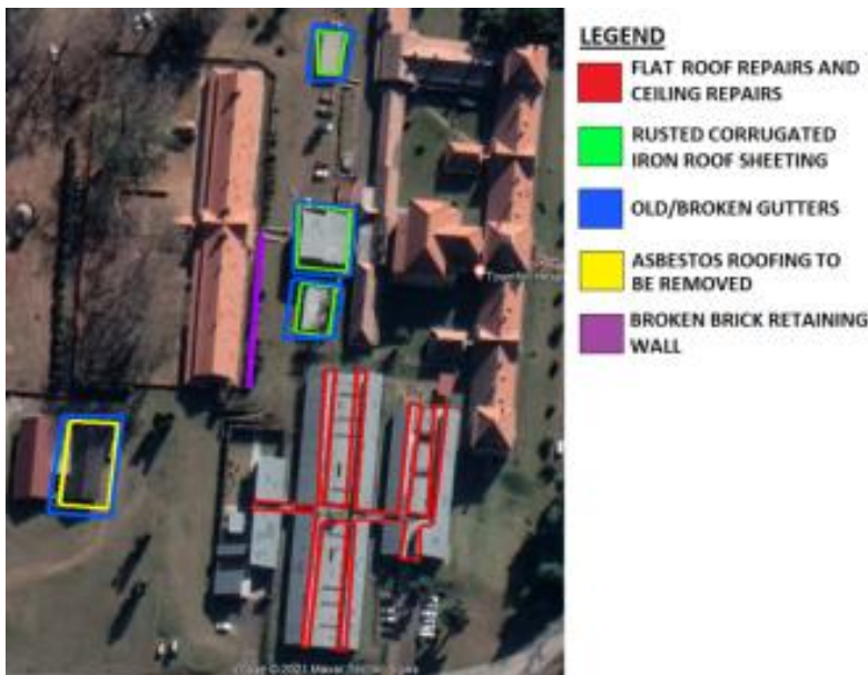
Figure 4: Site findings at the Impala building and adjacent parking areas
