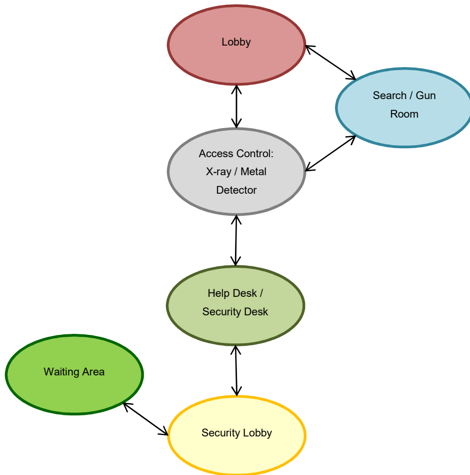
Figure 3: Unit Configuration for the main entrance
