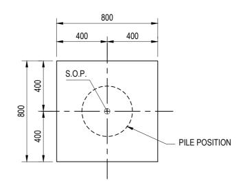
PILE DESIGN NOTES: ALL PILES TO BE DESIGNED TO TAKE MAXIMUM OF 800kN LOAD UNDER SERVICEABILITY LIMIT STATE. 2. ALL PILES TO BE FRICTION PILES. 3. ALL TOP OF PILE LEVELS TO BE VERIFIED AND CONFIRMED BY THE PROJECT CONTRACTOR.
